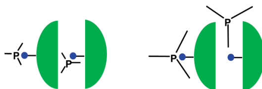
Figure C1-7. Schemes of the interaction of small-size (left-hand side) and large-size (right-hand side) probe molecules (e.g. alkylphosphines) with anchored metal sites (●) inside and outside the pores of a support material (◐◑). The ^{31}\text{P} nuclei of the adsorbed molecules are utilized as NMR probes.
